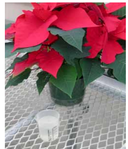
Figure 4. The goal for the PourThru test is to collect a leachate sample of approximately 50 milliliters (1.5 ounces).
