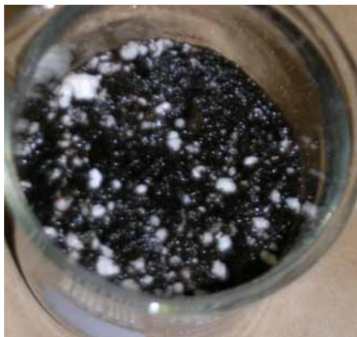
Figure 5. When using the saturated media extract method, the substrate should be saturated, but no free water should be visible on the sample surface.
